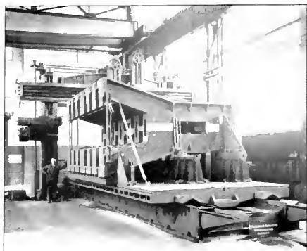
Group of A-frames on huge planer at the shops of the McIntosh & Seymour Corporation. This illustration gives an excellent idea of the size of castings.
